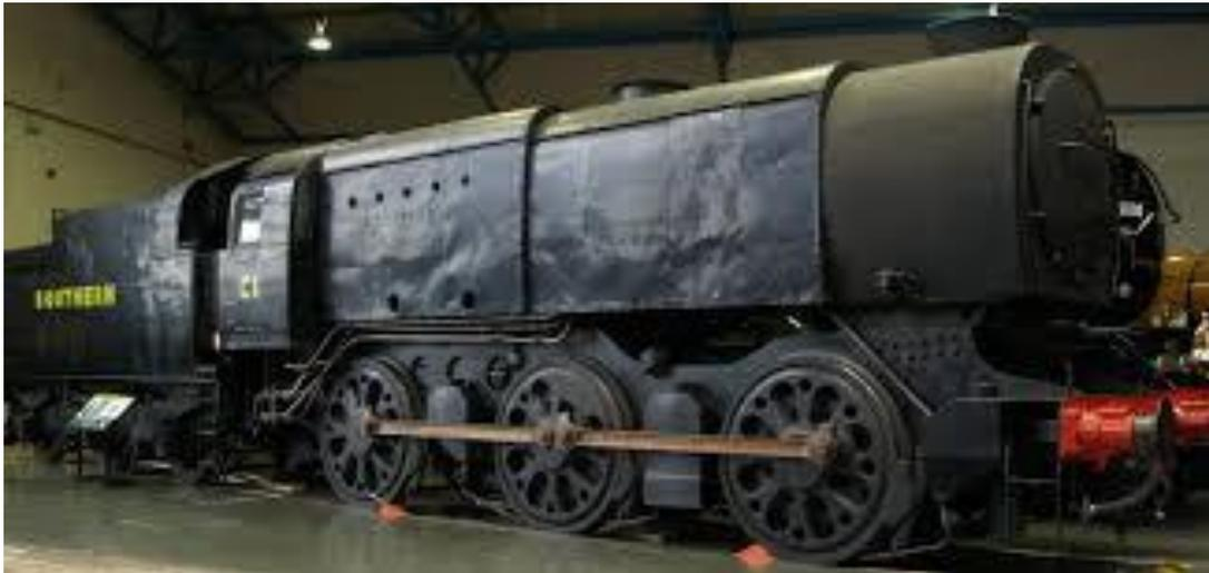
The second JTT locomotive kit is OVS Bulleid's Q1 0-6-0 tender engine. A wartime introduction, the Q1 was designed to produce a powerful locomotive with maximum route availability. Its unconventional appearance (Sir William Stanier is said to have remarked "Where does the key go?") was quite striking.
